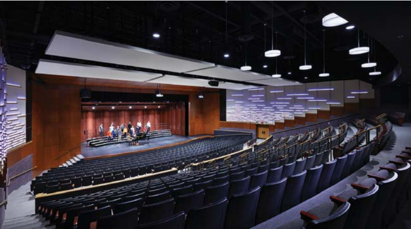
Proscenium theater with small thrust and steep rake at Mound Westonka High School in Minnetrista, Minn. Wold Architects & Engineers
