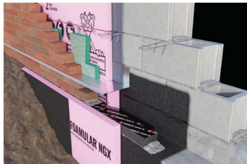
FOAMGLAS® Perinsul® SIB at the base of a masonry veneer exterior wall creates a continuous thermal barrier.
